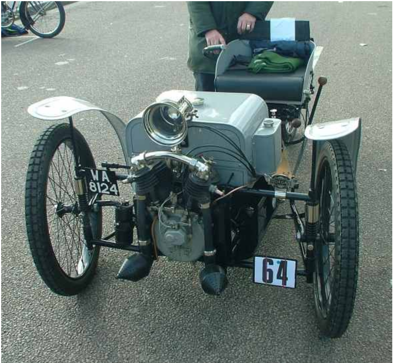
The 1909 Morgan again, this time a front view showing the 670cc P F (Peugeot) engine. I love the 'pepper pot' silencers.
