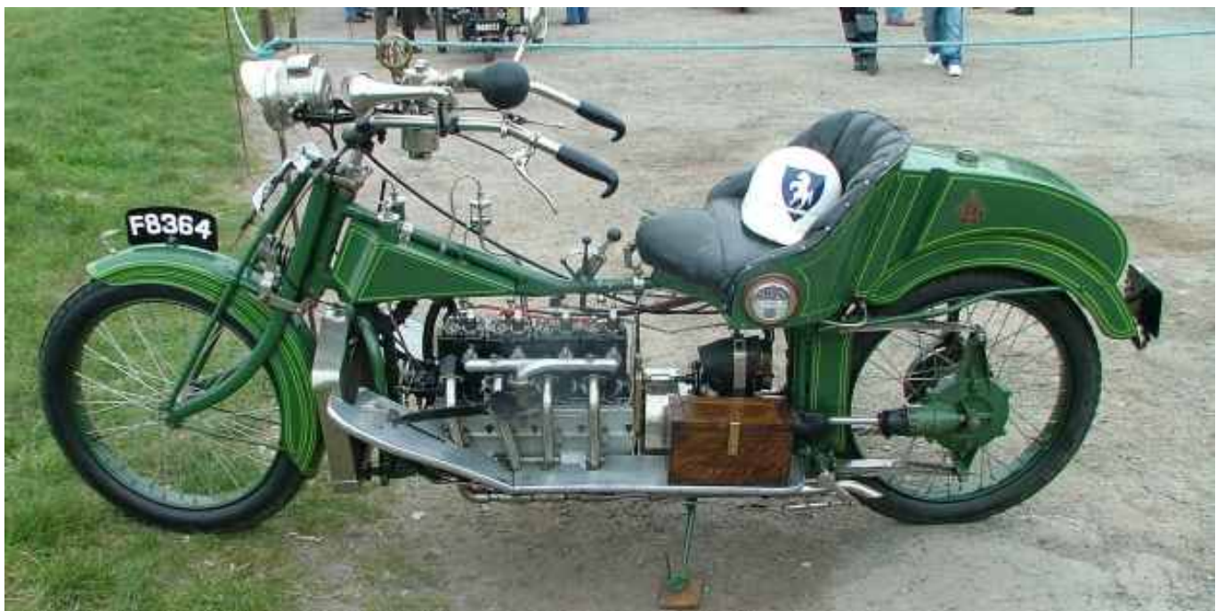
1913 Williamson 830cc inline four cylinder engine with water cooling & shaft drive.
