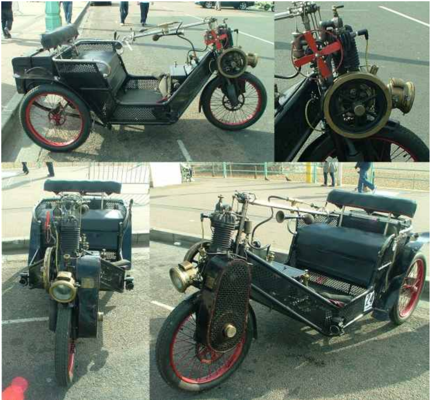
This wonderfully 'Heath Robinson' looking machine is a German Cyklon from 1903, powered by a 3.5HP single cylinder engine.
