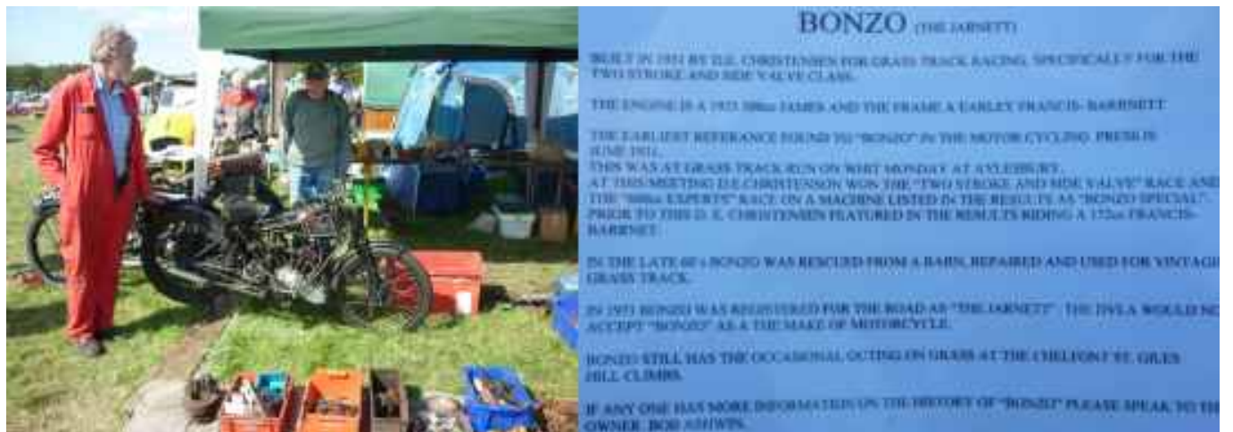
Andy's found a really interesting machine. A James vee twin side valve engine in a Francis Barnett frame.
