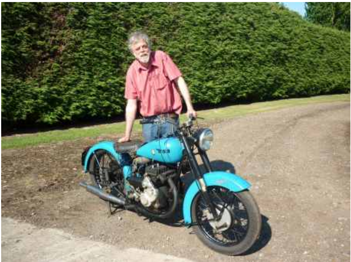
Andy showing off one of his more unusual machines, an air cooled Austin seven engined BSA.
